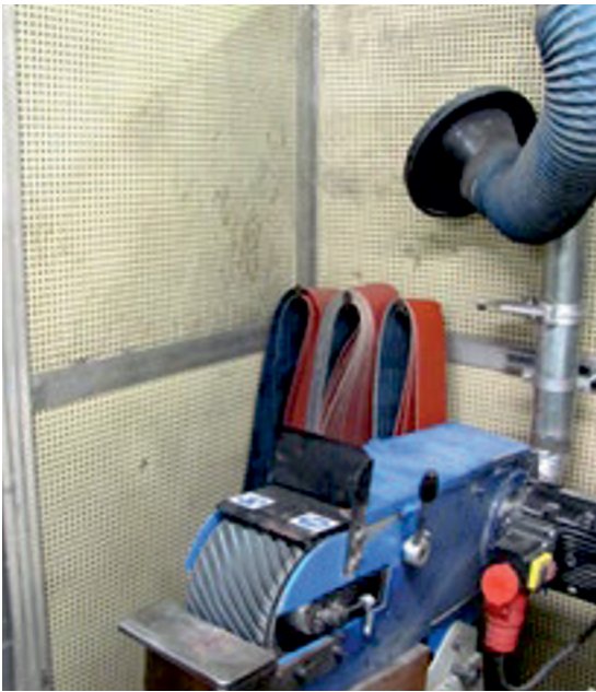
Figure 13 Movable acoustic screen in a foundry
