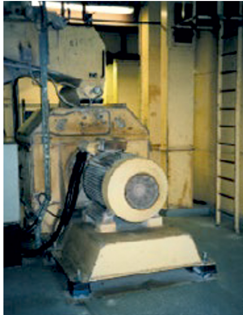
Figure 6 Vibration-isolating mounts reduce vibration entering the floor
