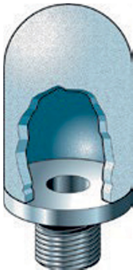
3c Injection-moulded plastic body and thread with sintered plastic or metal membrane
