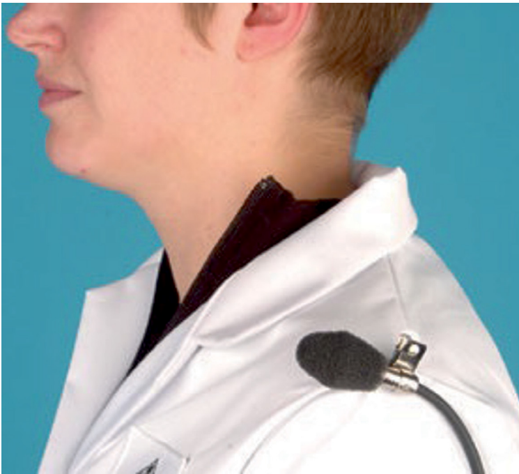
Figure 24 Recommended position for a dosemeter microphone
