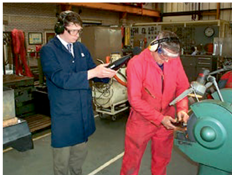
Figure 23 Making measurements with a hand-held sound level meter
