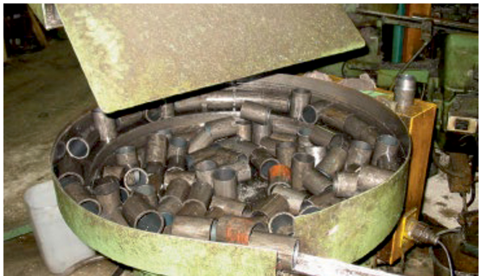
Figure 4 Reduced drop heights to reduce noise
